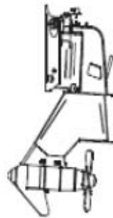
Type 2000B 288 hp @ 2300 rpm
