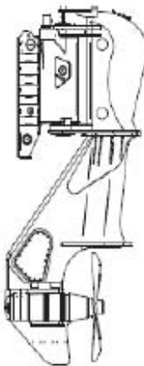
Type 4500B 536 hp @ 1800 rpm
